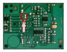
It is possible to supply the eLR1-868 receiver with a voltage of 12V. To do this, connect the solder points marked with the letter "A".
